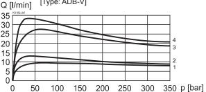
$\Delta p = f(Q)$ Pressure loss/flow characteristics (s = 100 %)
