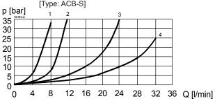
Volume flow-signal-characteristics ( $\Delta p = 10 \text{ bar}$ ) Q = f(s, x)[Type: ACB-S]
