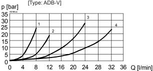
Q = f (s, x) Volume flow-signal-characteristics ( $\Delta p$  = 10 bar) [Type: ADB-V]
