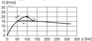
Q = f (p) Volume flow pressure characteristics [Type: S4D41-04] S = 100 %
