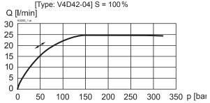
Q = f (s, x) Volume flow-signal-characteristics ( $\Delta p$  = 10 bar) [Type: V4D42]
