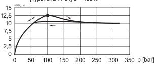
Q = f (s, x) Volume flow-signal-characteristics ( $\Delta p$  = 10 bar) [Type: S4D41]
