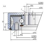
The mounting structure must support the housing to at least ø343 and at most to ø449
