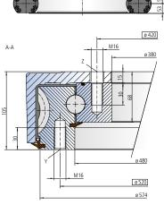
The mounting structure must support the housing to at least ø478
