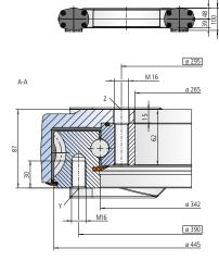
The mounting structure must support the housing to at least ø343 and at most to ø465
