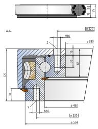
The mounting structure must support the housing to at least ø478
