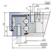
The mounting structure must support the housing to at least ø419 and at most to ø544
