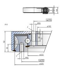
The mounting structure must support the housing to at least ø223 and at most to ø329
