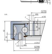
The mounting structure must support the housing to at least ø230 and at most to ø329
