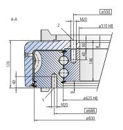
The mounting structure must support the housing to at least ø620 and at most to ø700
