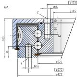
The mounting structure must support the housing to at least ø223 and at most to ø329
