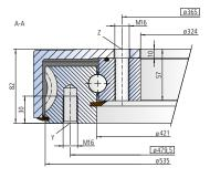
The mounting structure must support the housing to at least ø419 and at most to ø544
