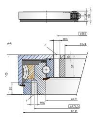
The mounting structure must support the housing to at least ø419 and at most to ø544
