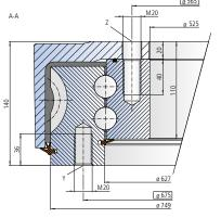
The mounting structure must support the housing to at least ø625
