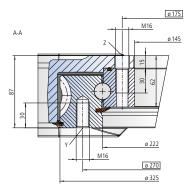
The mounting structure must support the housing to at least ø223 and at most to ø345
