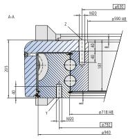
The mounting structure must support the housing to at least ø713 and at most to ø760
