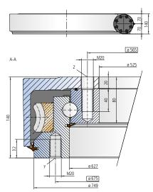
The mounting structure must support the housing to at least ø625
