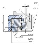
The mounting structure must support the housing to at least ø620 and at most to ø700
