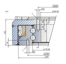
The mounting structure must support the housing to at least ø713 and at most to ø760
