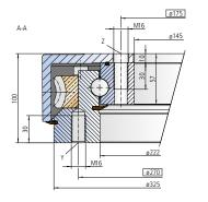
The mounting structure must support the housing to at least ø223 and at most to ø329
