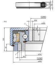
The mounting structure must support the housing to at least ø343 and at most to ø449
