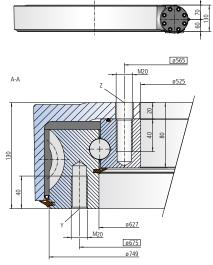
The mounting structure must support the housing to at least ø625
