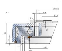
The mounting structure must support the housing to at least ø419 and at most to ø486
