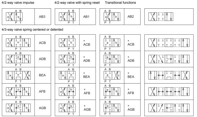
On all 4/2-way valves with spring reset the spring side must be connected to a tank or drain line.
