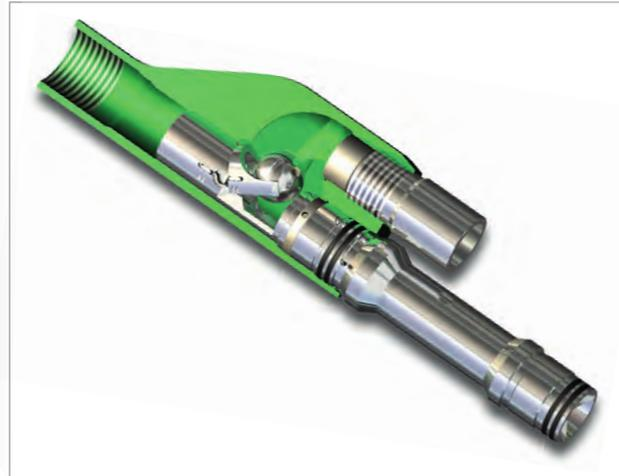
The Y-Chek, which features an internal travelling ball, is automatically activated by the flow and pressure produced by the downhole pump. The ball starts off in the flow path of the pump and will lift up and move over to the sealing position on the bypass tubing side upon pump start up. The pressure generated by the pump will keep the ball sealed in the seat position while the pump is running.
