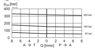
$p_{min} = f(Q)$ Minimal pressure loss/flow characteristics
