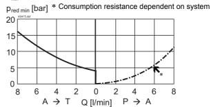
$\Delta p = f(Q)$  Pressure loss/flow characteristics over RV
